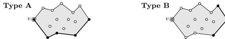
Fig. 11. The two types of pointgons we encounter in the first combined algorithm. A black point indicates a vertex belonging to V_p , a white point a vertex belonging to V_h , a grey point a vertex either in V_p or in V_h . The encircled point is the anchor. Thick lines indicate pieces of the perimeter of the input pointgon.
